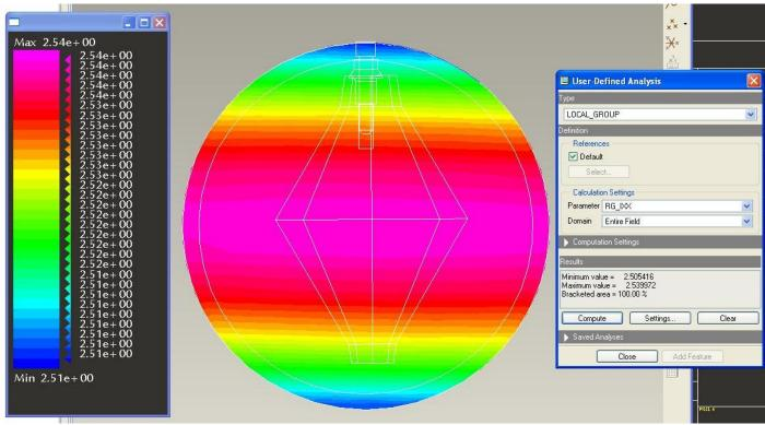
Figure 1: Generic Lane #1 Diamond Core w/ Plotted Rg Contours
