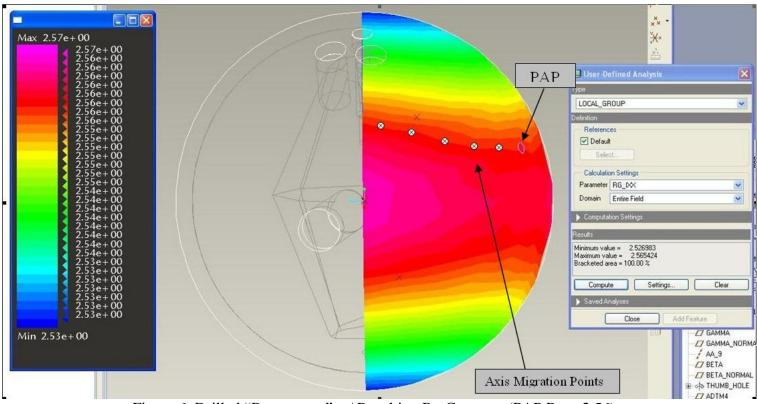
Figure 6: Drilled "Boomerang" w/ Resulting Rg Contours (PAP Rg = 2.56)
